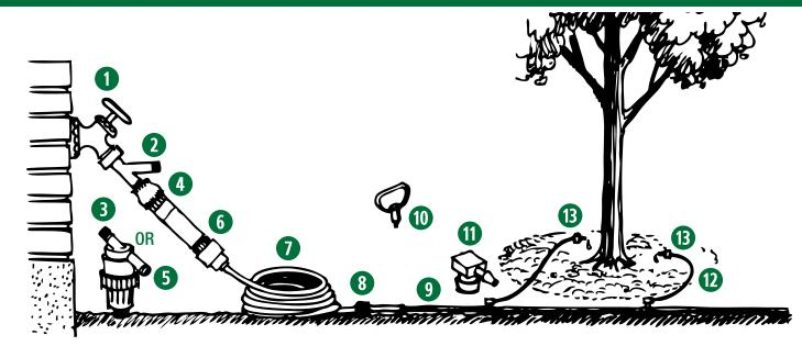
Connect your system to any OUTDOOR FAUCET. Knowing the delivery rate of the emitters (13), the water needs of your trees, and the kind of soil you have (clay requires more watering time than loam or sandy soil), you can open the valve for the necessary length of time during dry periods. Automatic timers can be inserted here.
