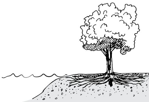
**DRAINAGE CHANGES** If terrain is altered, there will be a change in how water drains from the land. If flows are created that add too much moisture to a wooded site, a drainage system may be needed to maintain the previous amount of moisture (which provided the natural growing conditions for the existing trees.) Similarly, existing trees along the edge of a new pond may eventually die from their roots suffocating. On sites deprived of water, irrigation may be needed to maintain existing trees.
