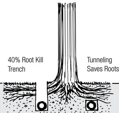
**SEVERING ROOTS** Some cutting of roots near construction is inevitable, but much is avoidable. For example, the routing of underground utilities does not have to follow a straight line from street to house. Careful route selection can often avoid important trees. When that is not possible, tunneling is a good way to reduce damage. To reduce trenching for foundations, posts and pillars can be substituted for footers and walls.
