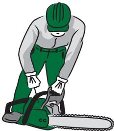
After selecting a safe area and checking for proper chain tension, oil and fuel, start the saw by holding the saw firmly against the ground with one hand on the front handle and placing a knee or foot on the rear handle. Give the starter rope a quick but short pull. Make choke adjustments as necessary.
