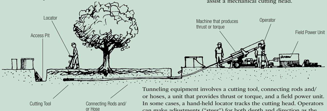
Tunneling equipment involves a cutting tool, connecting rods and/or hoses, a unit that provides thrust or torque, and a field power unit. In some cases, a hand-held locator tracks the cutting head. Operators can make adjustments (“steer”) for both depth and direction as the tunneling proceeds. Accuracy of some methods is within inches of a target (usually an access pit) at the end of the tunneled span.
