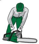
After selecting a safe area and checking for proper chain tension, oil and fuel, start the saw by holding the saw firmly against the ground with one hand on the front handle and placing a knee or foot on the rear handle. Give the starter rope a quick but short pull. Make choke adjustments as necessary.
