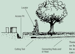
Tunneling equipment involves a cutting tool, connecting rods and/ or hoses, a unit that provides thrust or torque, and a field power unit. In some cases, a hand-held locator tracks the cutting head. Operators can make adjustments ("steer") for both depth and direction as the tunneling proceeds. Accuracy of some methods is within inches of a target (usually an access pit) at the end of the tunneled span.
