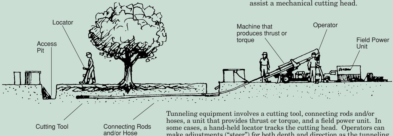
Tunneling equipment involves a cutting tool, connecting rods and/or hoses, a unit that provides thrust or torque, and a field power unit. In some cases, a hand-held locator tracks the cutting head. Operators can make adjustments (“steer”) for both depth and direction as the tunneling proceeds. Accuracy of some methods is within inches of a target (usually an access pit) at the end of the tunneled span.
