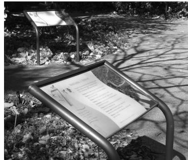
The interpretive signs are silk-screened on 30-by-18-inch panels. Illustrations and text are used to help viewers understand the xeriscape principles being demonstrated and to identify woody plants. Three-inch, grey micarta labels on stands supplement the interpretive signs by identifying herbaceous plant materials.
