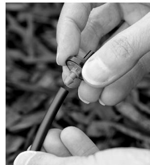
For trouble-free operation, be sure to use emitters that are self-flushing to prevent clogging and pressure-compensating so the rate of drip does not vary due to distance from the water source.
