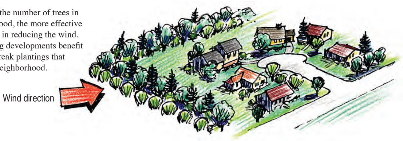
A well-placed windbreak can protect several homes or an entire development from chilling winter winds and drifting snow.
